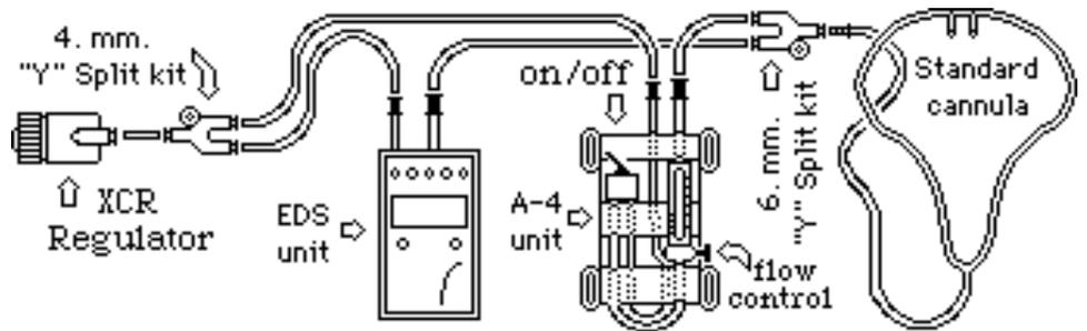
Because many pilots fly with passengers only part of the time, the A-3 or A4 flowmeter/regulator and an Oxyimizer® cannula can be setup for the bypass station and for the passenger.
