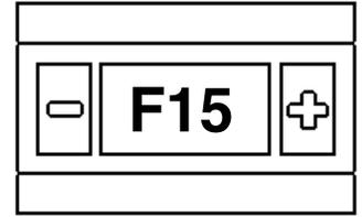
Switch as seen in the Floor mode. The F15 setting provides 15,000 ft. amount of oxygen referenced to sea level or that respective additional amount throughout the pressure altitude curve
