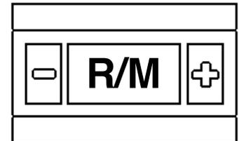
Switch as seen in the Reserve/Manual setting. 100% delivery or for use with regulators that are flow-rate adjustable.
