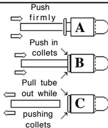
*To remove the polyurethane service line you must push in the connector collar while you pull on the polyurethane line. Do not pull the polyurethane line without pushing in the collar. It will damage the connector rendering it useless.*
