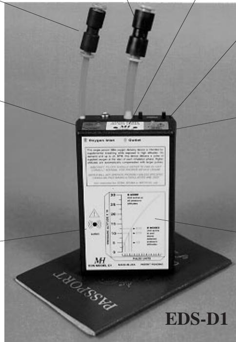
Up to (8) eight EDS-D1 units can be powered from our optional EPS (External Power Supply) unit if it is desirable to use the power system from an aircraft. The EPS is a 10 volt @ 500 ma. low-drop-out voltage regulator and filter unit that operates from 11 to 28 volts. It filters out glitches caused by hydraulic pumps, strobe lights and other high-energy devices. It works
