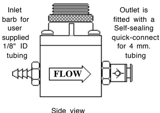
**The EDS regulator stabilizer unit is designed to allow up to six EDS units to be operated from a built-in oxygen system where the pressure is 20 to 125 psig. thus replacing the standard issue XCR regulator.**
